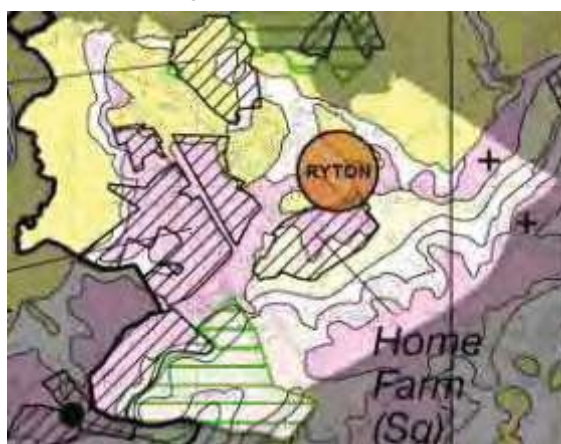
Figure 7: Ryton extract from Mineral Resources map (British Geological Survey, for Warks CC); Pink = sand and gravel. Hatched = worked out
